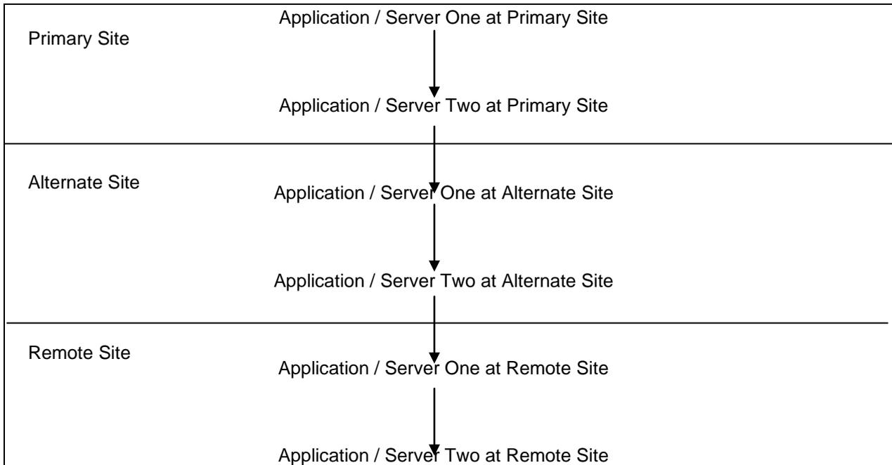
Intra-site failover will be transparent to the end user and connectivity will not be impacted. During an inter-site failover, all connectivity is lost, and participants must log in to re-establish a communication link. All three Sites utilize the same IP address and ports. Therefore, participants only need to retain a single IP address for the Primary, Alternate and Remote Site.
