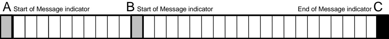
When a Start of Message indicator (B) appears after the true Start of Message (A) and before the End of Message indicator (C), the bytes from A to B are discarded, and a message is written to the internal error log. The bytes from B to C are sent to the message processor for edit checking.
